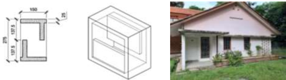
Figure 5. Ventilation block used in the case study cottage and the location of brise soleil and vent blocks below the roof on the western wall of the living room. (Source: Authors)
