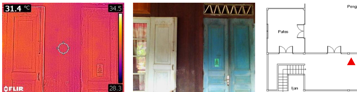
(a) Surface temperature of outside wall (facing South)
